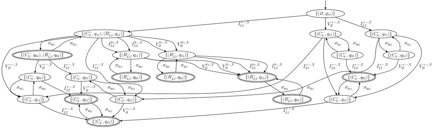
Fig. 3. Partial hybrid diagnoser for  $F = \{C_0^-, R_{L1}^-\}$  and initial mode  $q_{11}$ .
