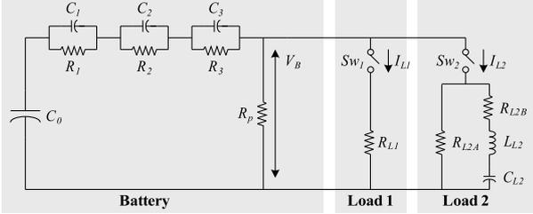
Fig. 2. Circuit equivalent for the selected subsystem.
