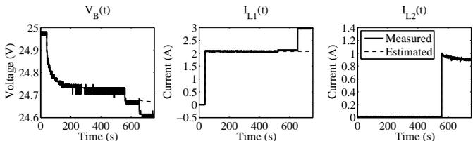
Fig. 5.  $R_{L1}^-$  fault, where  $R_{L1}$  decreases by 33%.
