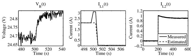
Fig. 4.  $R_{L1}^-$  fault, where  $R_{L1}$  decreases by 33% followed by  $\sigma_{q_{01}}$ .
