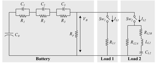
Figure 2: Electrical circuit equivalent for the selected subsystem.
