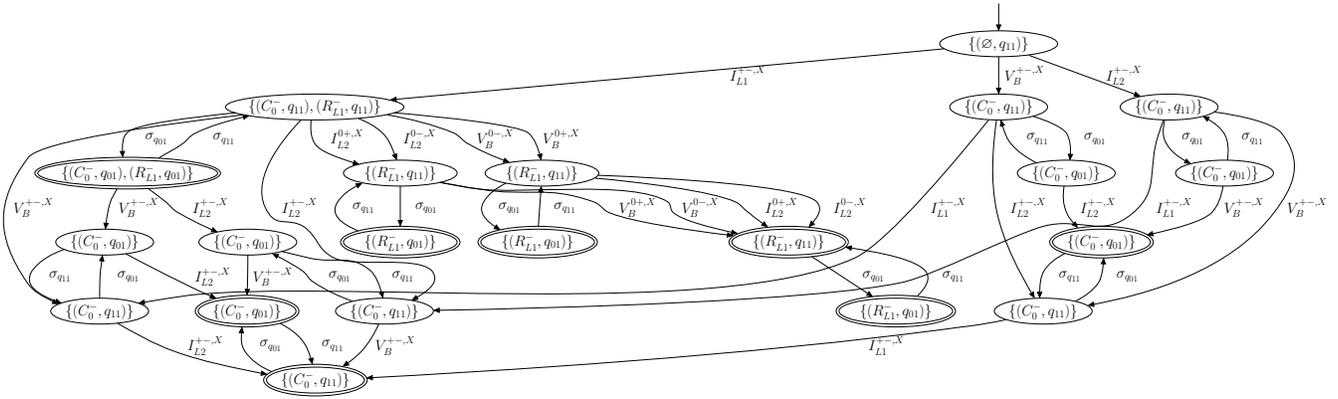
Figure 5: Partial hybrid diagnoser for  $F = \{C_0^-, R_{L1}^+\}$  and initial mode  $q_{11}$ .
